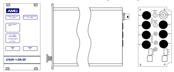
The AMG2783R-1-DR-SF is a single channel video insert unit designed to transmit a video signal on to a single dual redundant optical fibre ring. It also provides a RS485/RS422 bi-directional data channel. It is designed to be mounted in an AMG2005 19" rackmount subrack.
